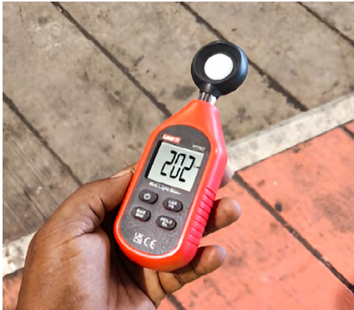
> Illumination of loading / unloading bay at Loghub
